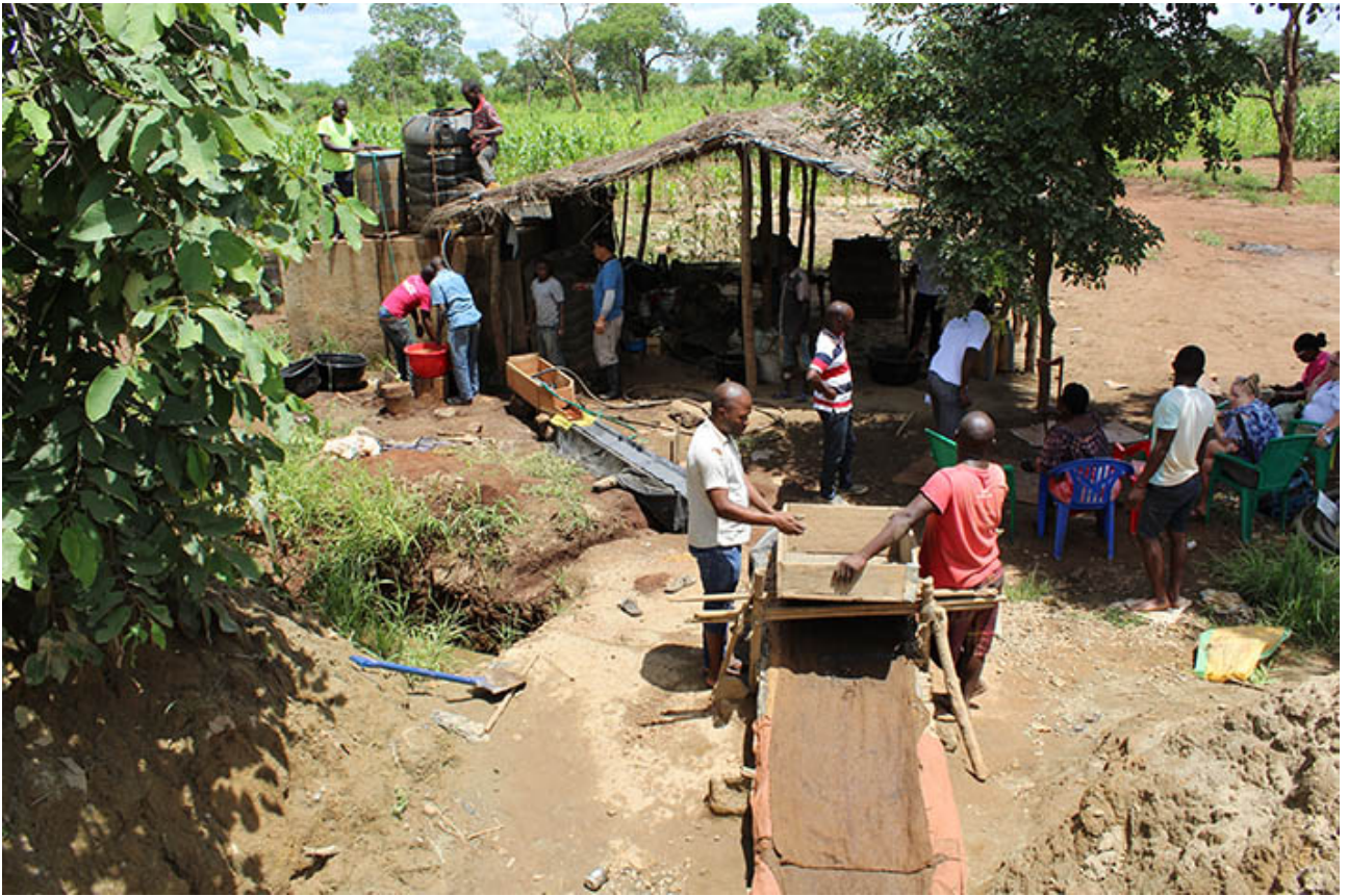
Old method using mercury in the foreground versus new mercury-free gold extraction in the background in Wacueia
