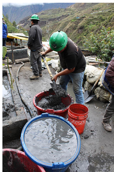
Fig. 8 Splitting sample to two tubs with and without organic
